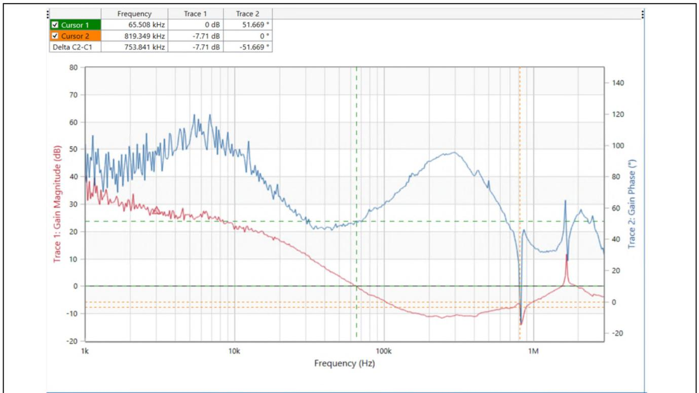
**Figure 17** Bode plot of the PXE1610C control loop with 130 A of constant load current
