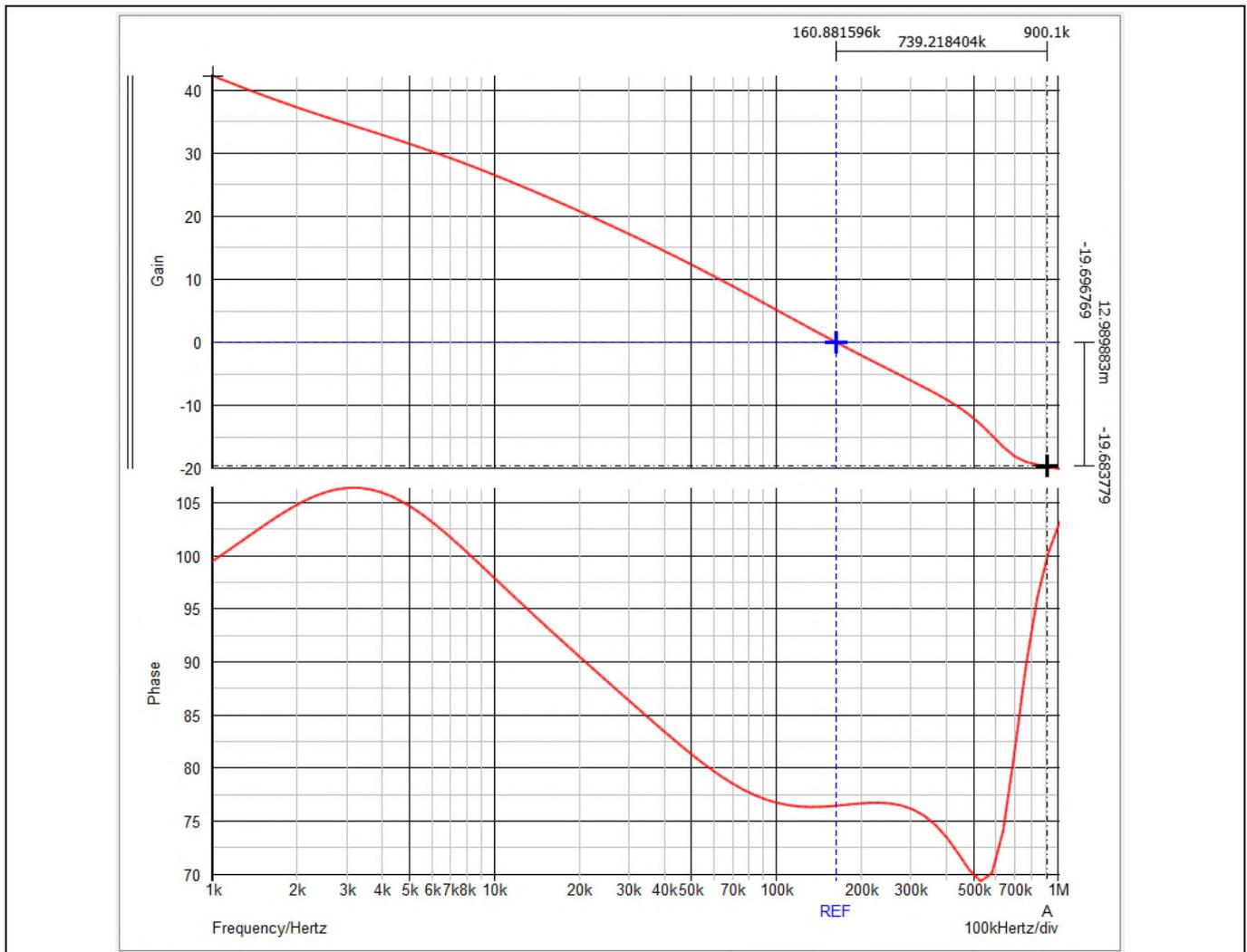
**Figure 13** Bode plot of the control loop with 97.5µΩ of LL
