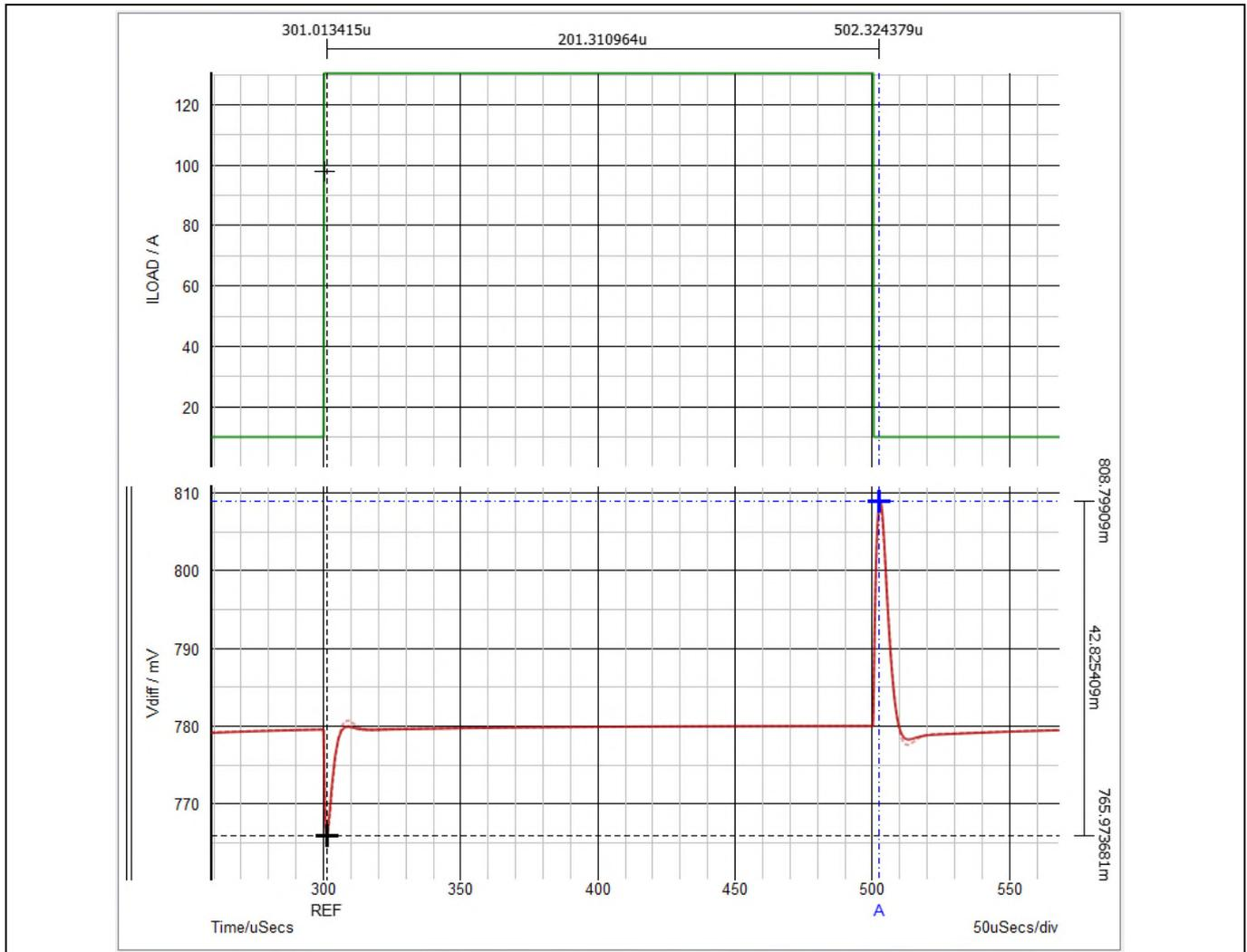
**Figure 4 Transient response of a six-phase buck converter without LL enabled**
