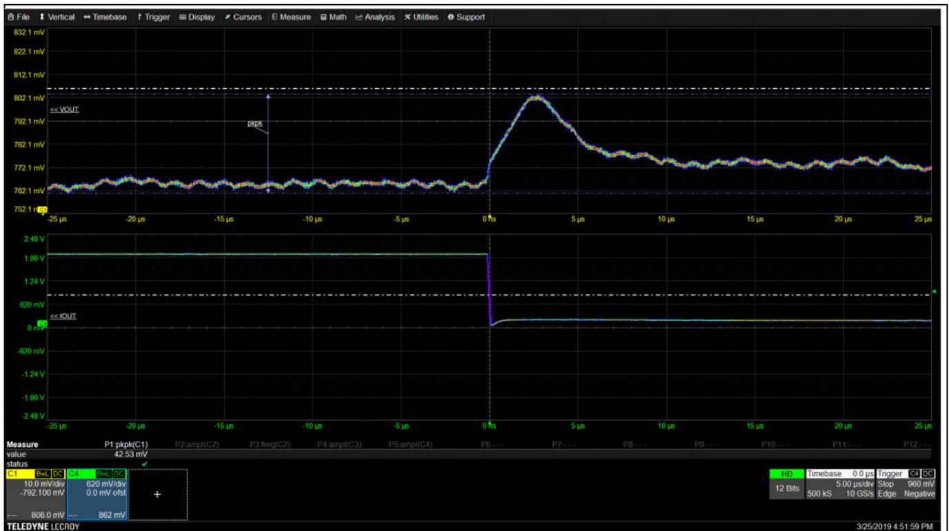
**Figure 16** Transient load release from 130 A to 10 A in 200 ns
