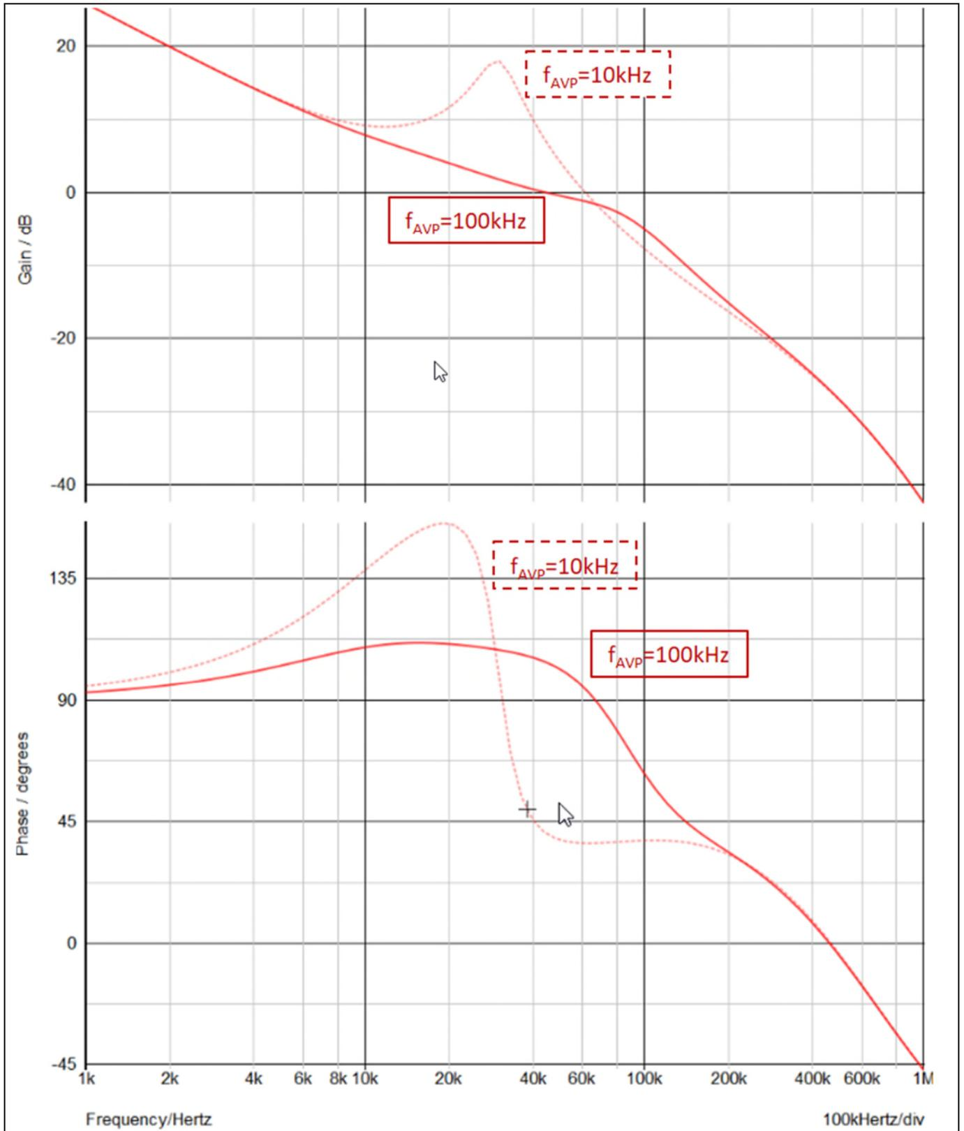
**Figure 11 AVP roll-off frequency impact on resonant spike**
