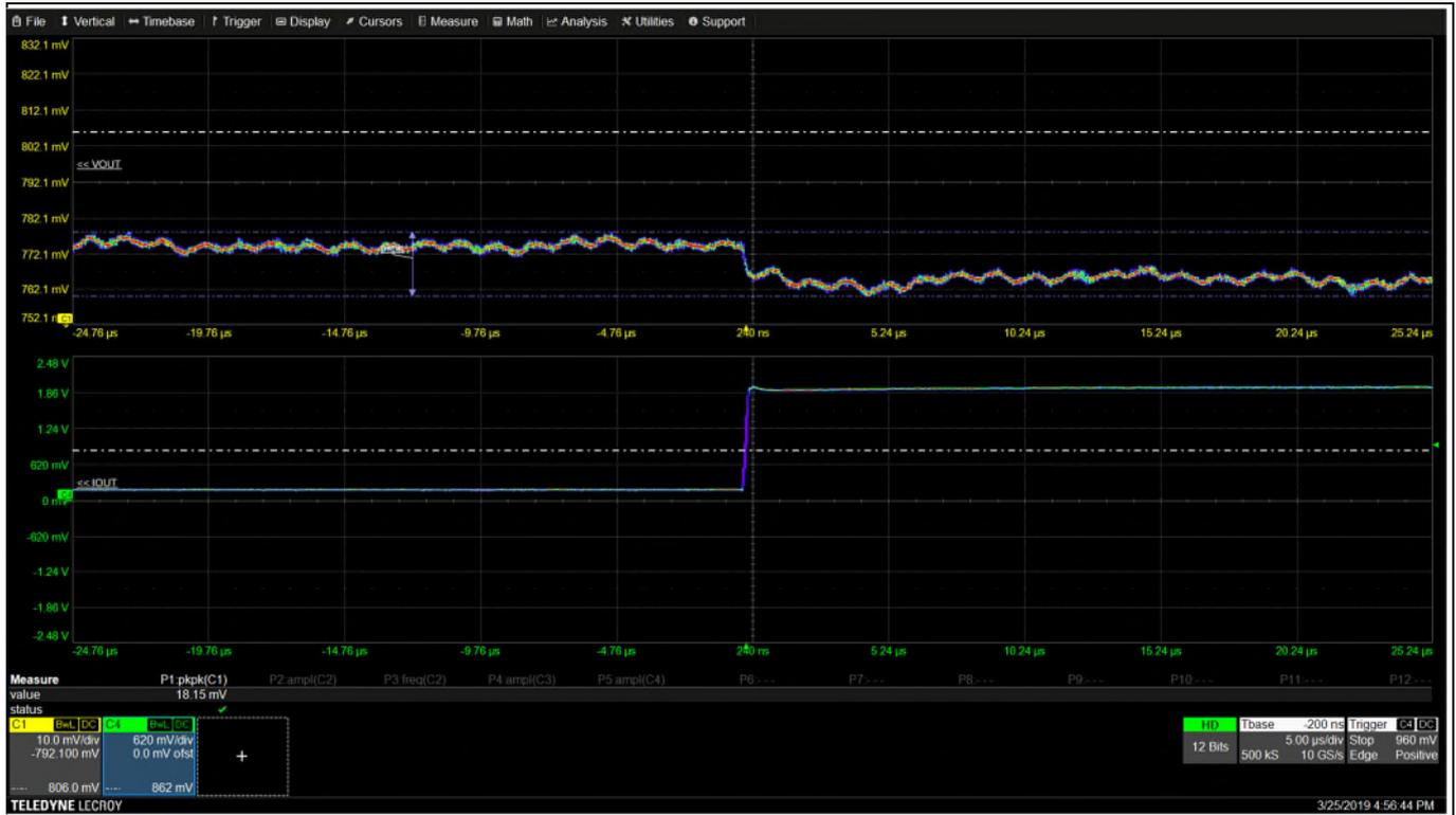
**Figure 15** Transient load step from 10 A to 130 A in 200 ns
