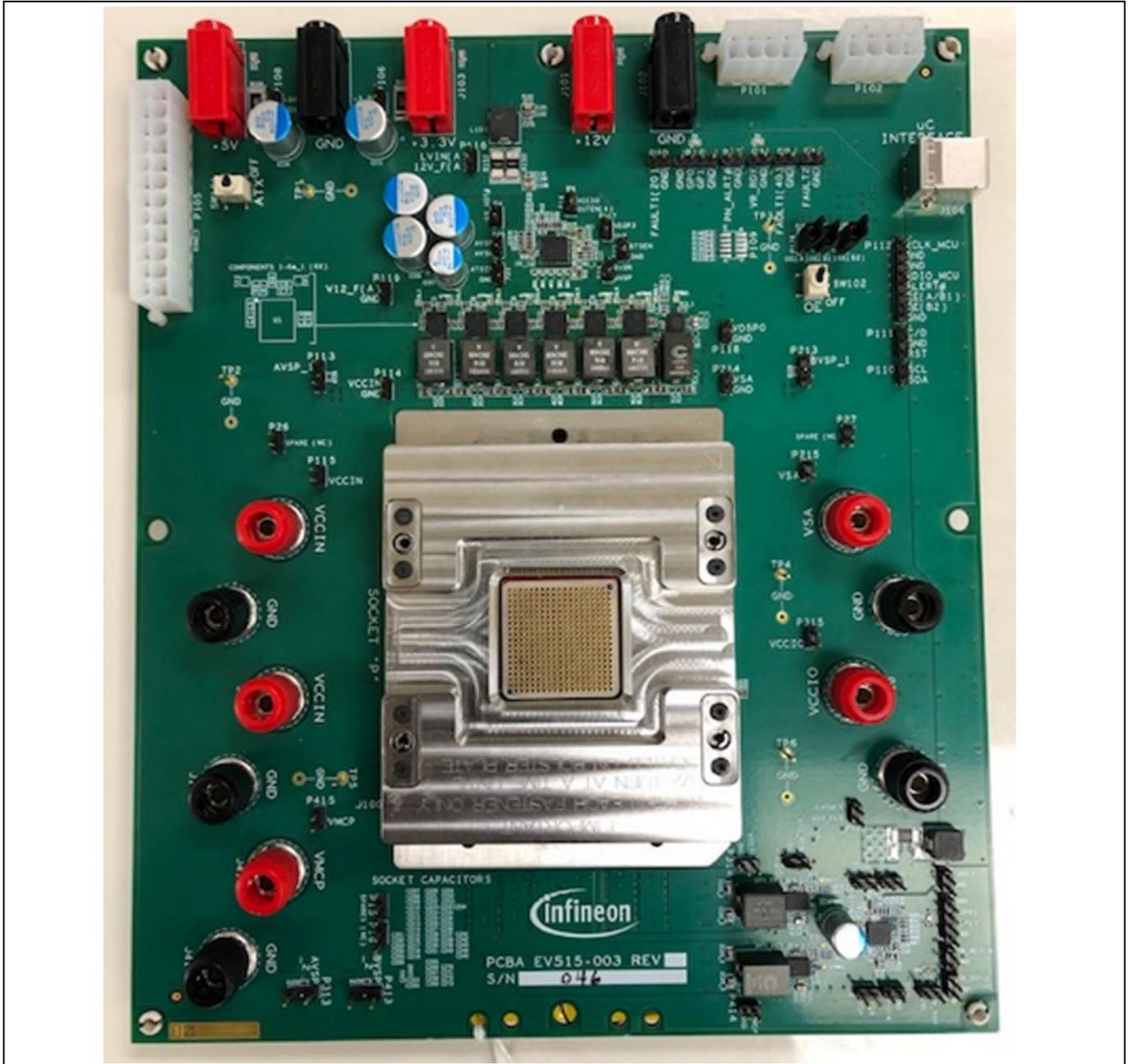
**Figure 3** Picture of the PXE1610C demo board used for hardware testing and verification
