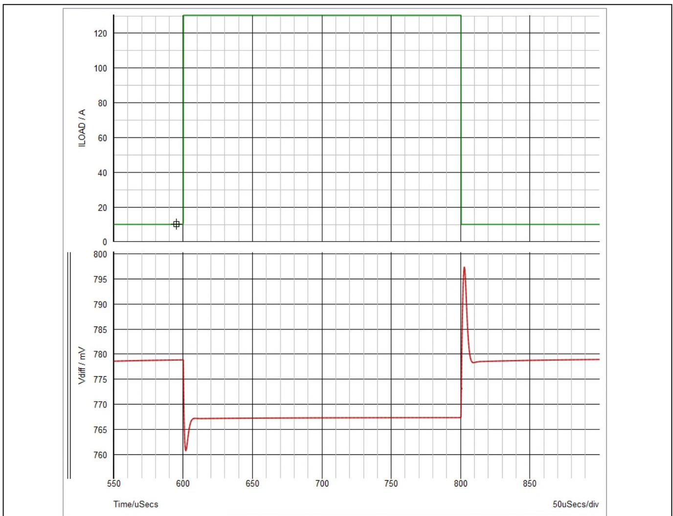
**Figure 12** Transient response with  $97.5\text{ }\mu\Omega$  of LL
