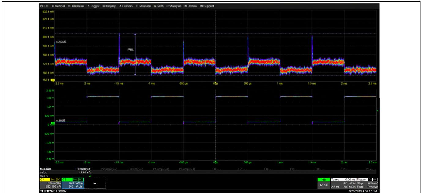
**Figure 14** Transient load steps and releases over multiple load cycles at a duty cycle of 0.5 and 1 kHz repetition rate
