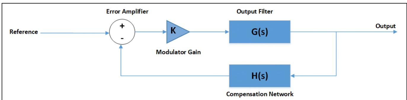
**Figure 8** Control loop of a voltage-mode buck converter
