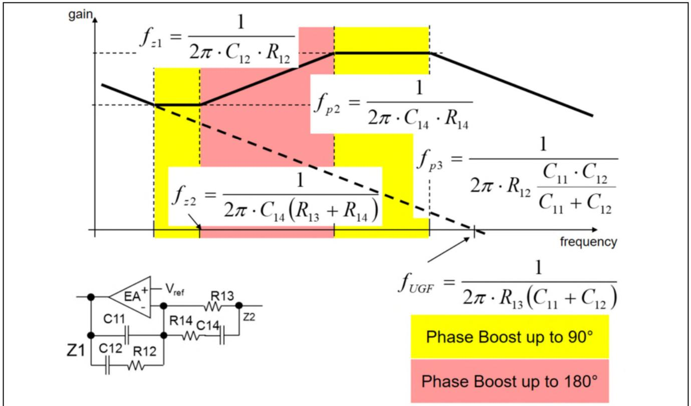
**Figure 6** PID compensation network with Type III analog error amplifier
