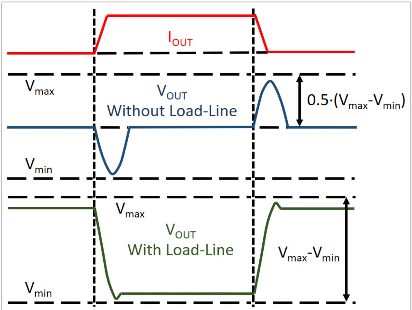
**Figure 2**  $V_{OUT}$  behavior during a transient event with and without LL
