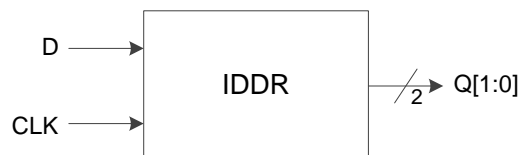
Figure 3-18 I/O Logic in DDR Input Mode
