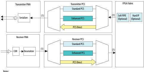
(1) The FPGA Fabric - PCS and PCS-PMA interface widths are configurable.
