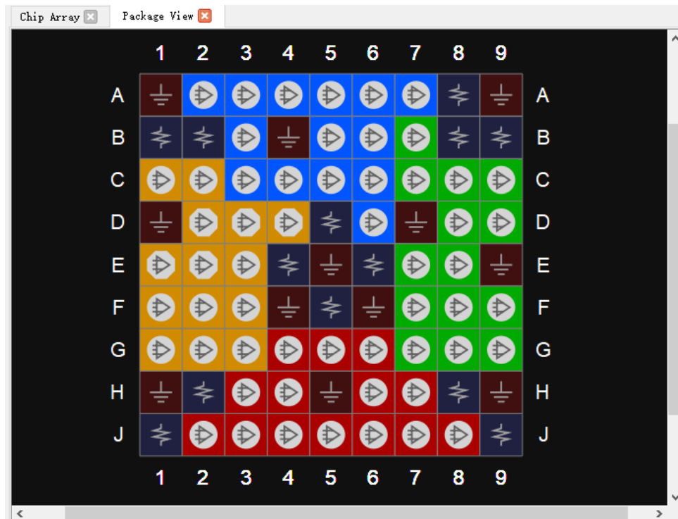
Figure 3-38 GW1N-9-WLCSP81M Bottom View
