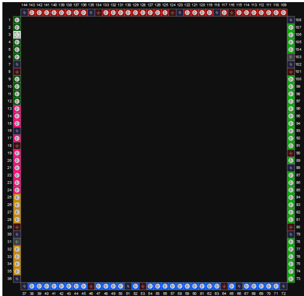
Figure 3-13 View of GW1N-2 LQ144 Pins Distribution (UV Version, Top View)
