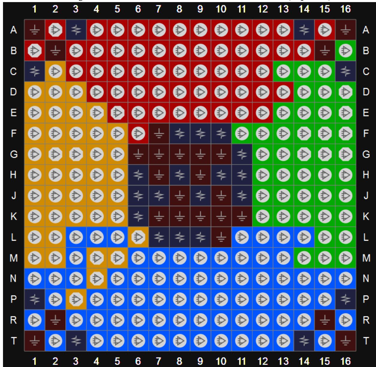
Figure 3-44 View of GW1N-4 PG256M Pins Distribution (Top View)
