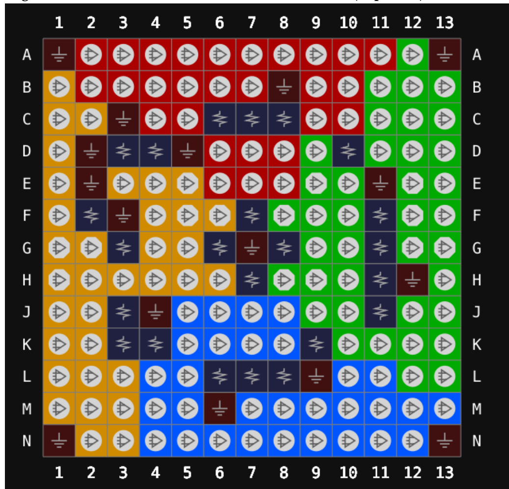
Figure 3-54 View of GW1N-9 UG169 Pins Distribution (Top View)
