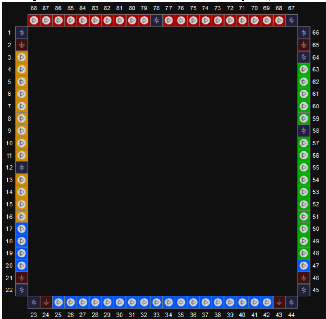
Figure 3-38 View of GW1N-4 QN88 Pins Distribution (Top View)
