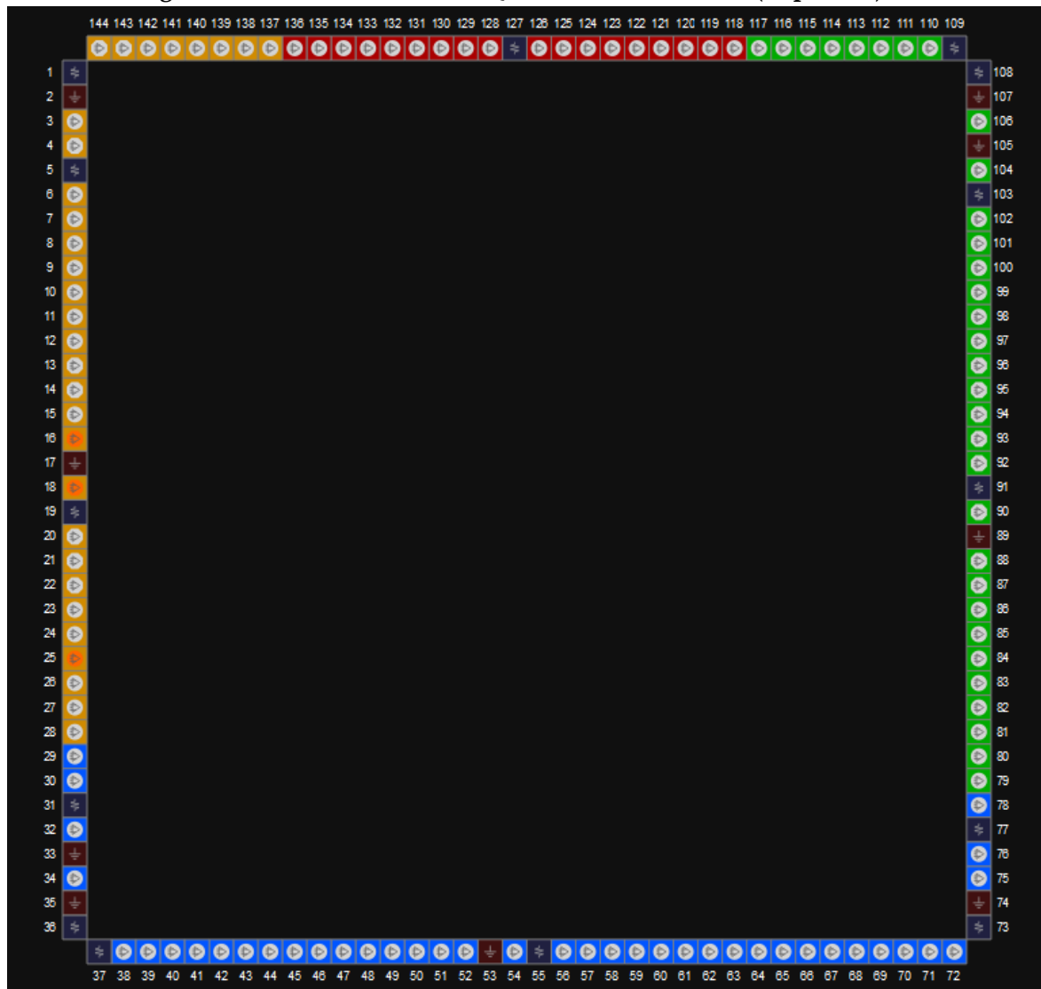
Figure 3-52 View of GW1N-9 EQ144 Pins Distribution (Top View)
