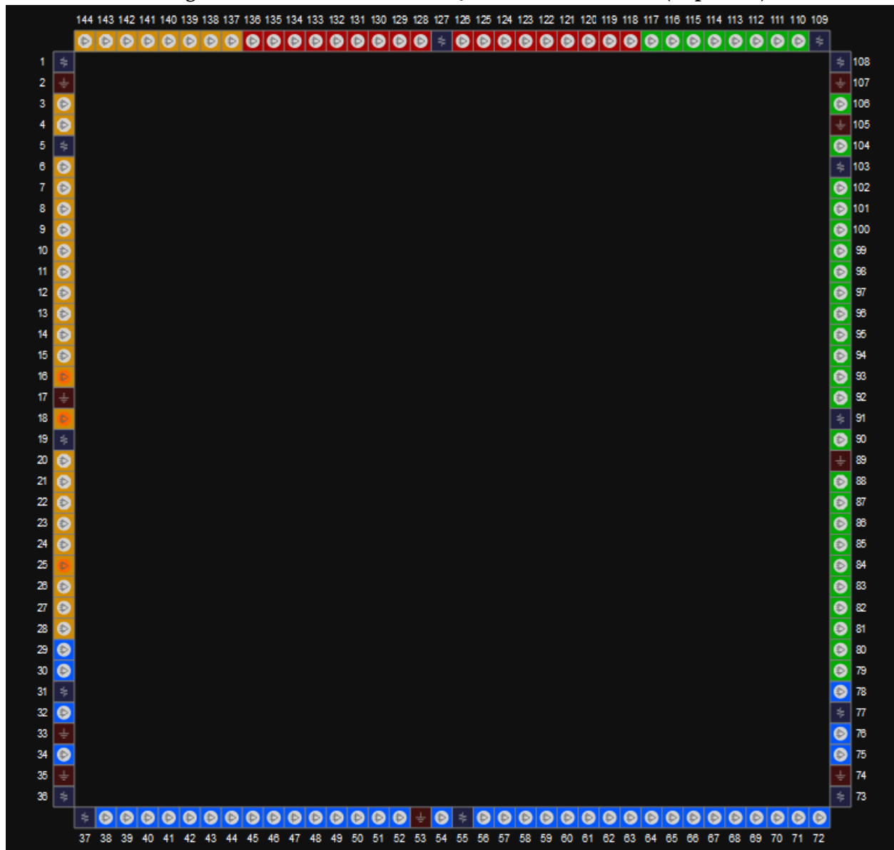
Figure 3-51 View of GW1N-9 LQ144 Pins Distribution (Top View)
