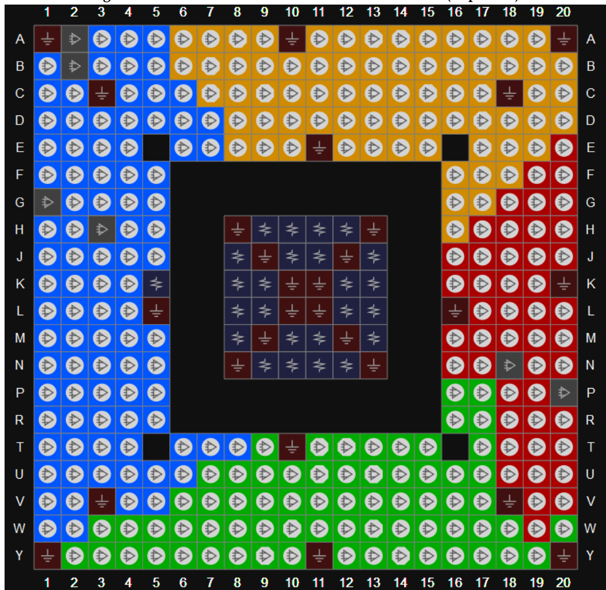
Figure 3-60 View of GW1N-9 UG332 Pins Distribution (Top View)
