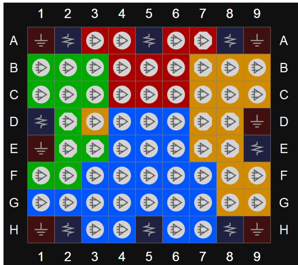
Figure 3-37 View of GW1N-4 CS72 Pins Distribution (Top View)
