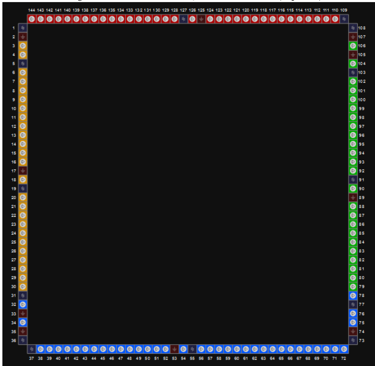
Figure 3-41 View of GW1N-4 LQ144 Pins Distribution (Top View)
