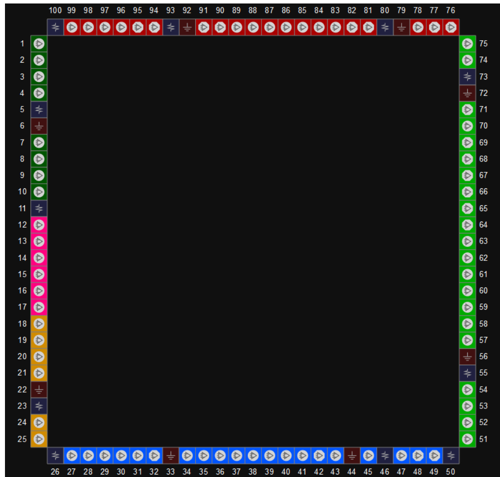
Figure 3-10 View of GW1N-2 LQ100 Pins Distribution (LV Version, Top View)
