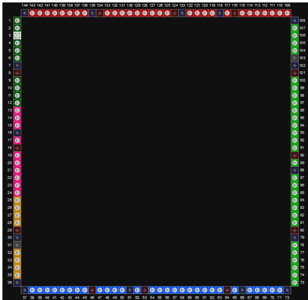
Figure 3-11 View of GW1N-2 LQ144X Pins Distribution (UV Version, Top View)
