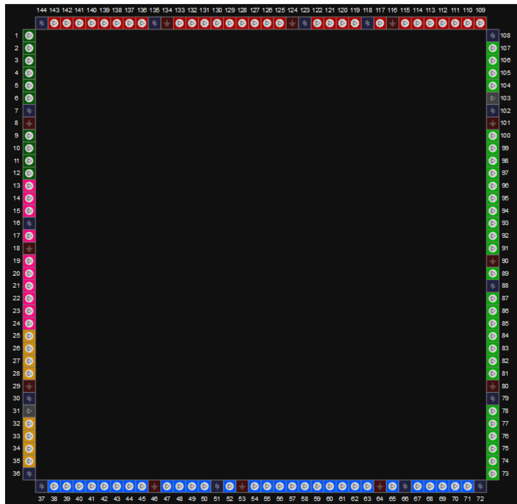
Figure 3-12 View of GW1N-2 LQ144X Pins Distribution (LV Version, Top View)
