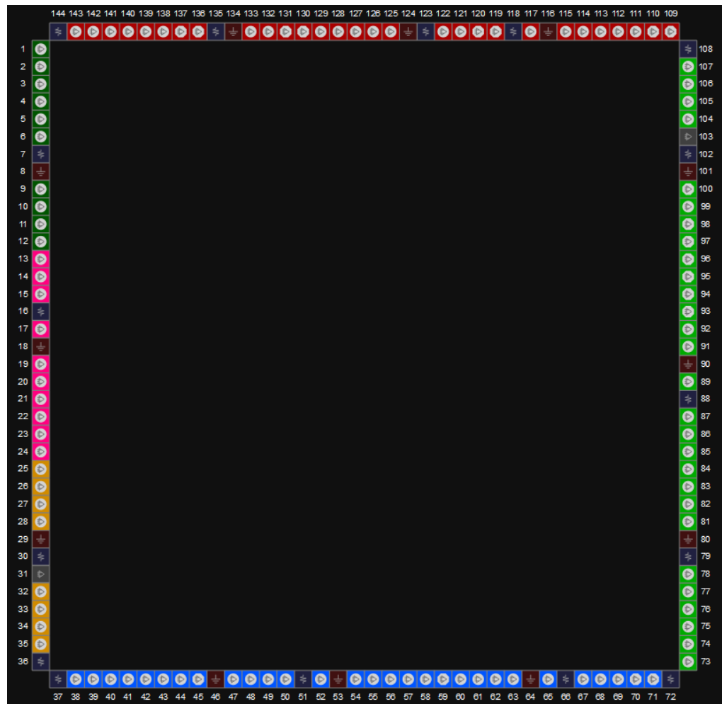
Figure 3-14 View of GW1N-2 LQ144 Pins Distribution (LV Version, Top View)
