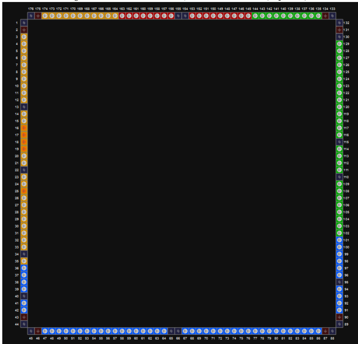
Figure 3-55 View of GW1N-9 LQ176 Pins Distribution (Top View)
