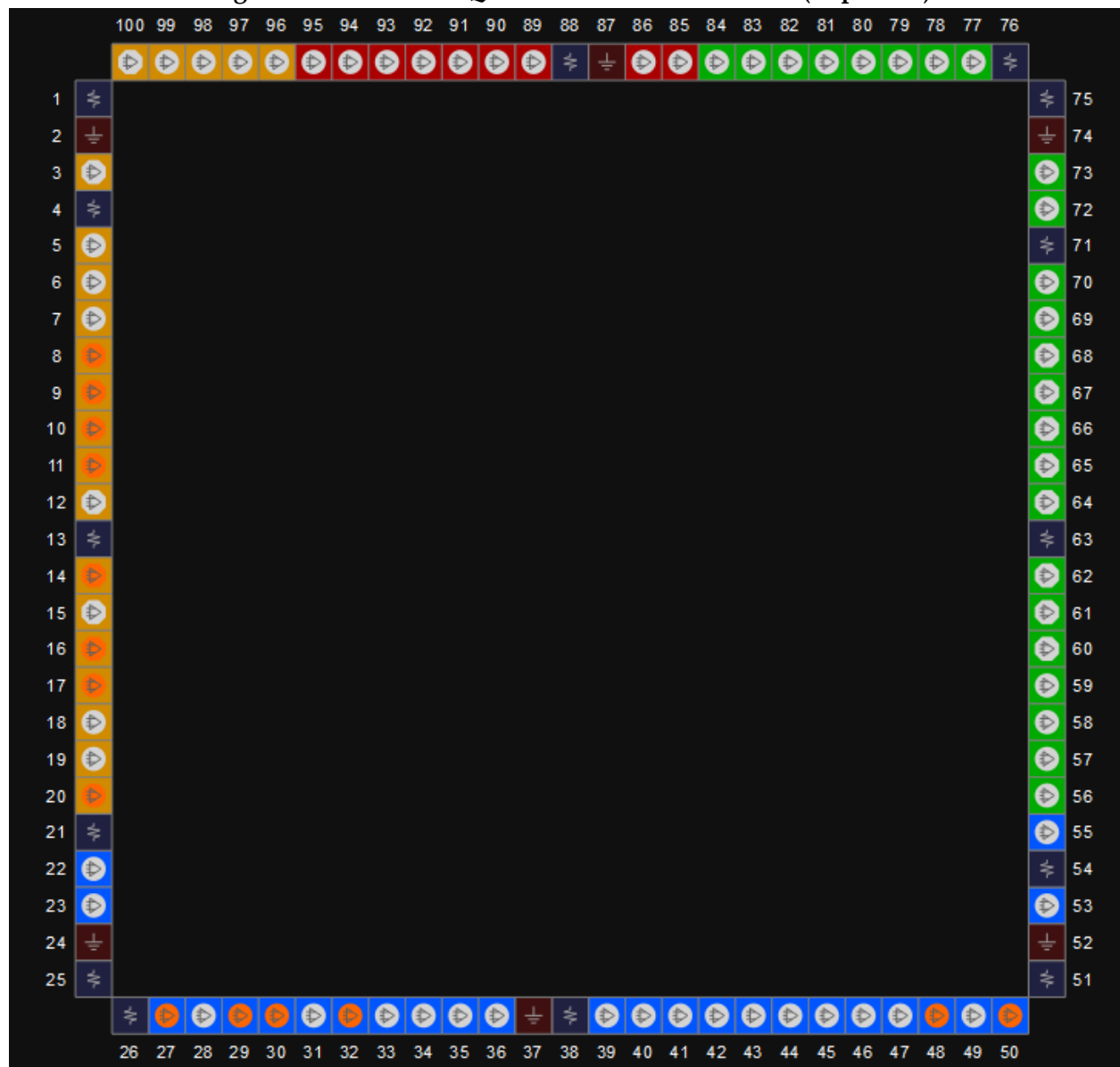
Figure 3-49 GW1N-9 LQ100 Pins Distribution View (Top View)
