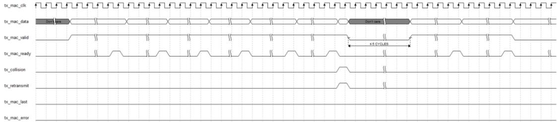
**Figure4-25 Abort Retransmission in case of Collision (Actively)**
