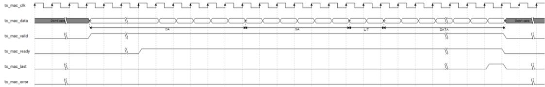
**Figure4-17 In RGMII Mode Normal Ethernet Frame Transmission at 10M/100M Rate**
