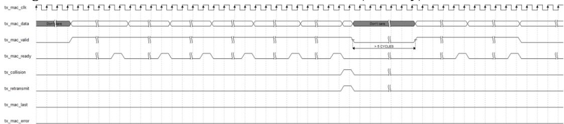
**Figure4-26 Abort Retransmission in case of Collision (Passively)**
