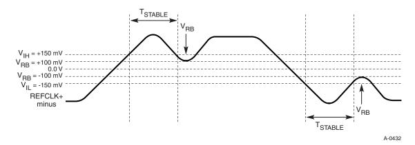
Figure 2-8: Differential Measurement Points for Ringback
