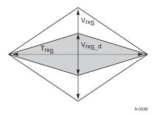
Figure 4-12: Representative Composite Eye Diagram for System Board Receiver Path Compliance
