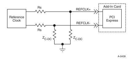
Figure 2-2: Example Reference Clock Source Termination
