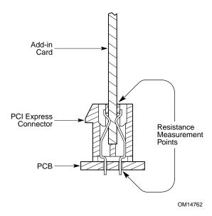
Figure 5-5: Contact Resistance Measurement Points
