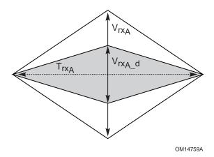
Figure 4-9: Representative Composite Eye Diagram for Add-in Card Receiver Path Compliance
