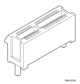
Figure 1-1: Vertical Edge-Card Connector
