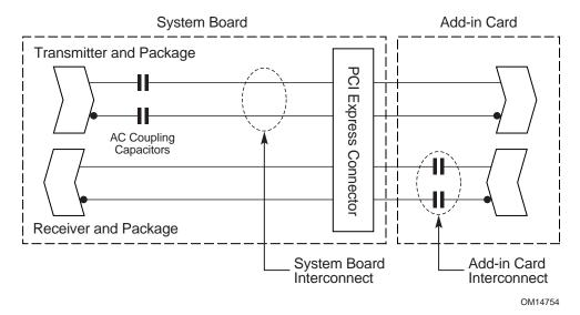
Figure 4-4: Link Definition for Two Components
