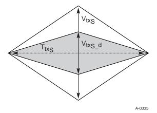
Figure 4-10: System Board Transmitter Path Composite Compliance Eye Diagram
