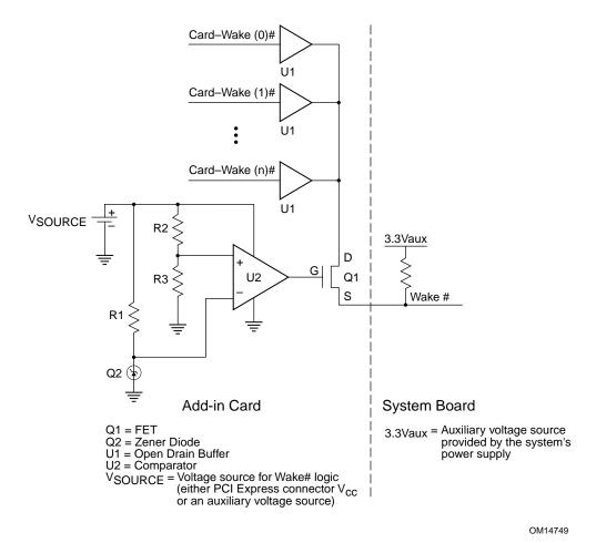
This example assumes that all sources of WAKE# on the add-in card are powered by either the +3.3V or +3.3Vaux ( $V_{SOURCE}$ ). If WAKE# from D3<sub>cold</sub> is supported by some, but not all of the add-
