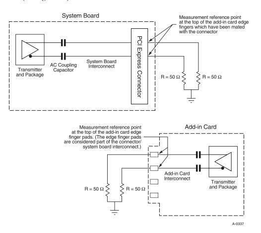
Figure 4-5: Example Interconnect Terminated at the Connector Interface
