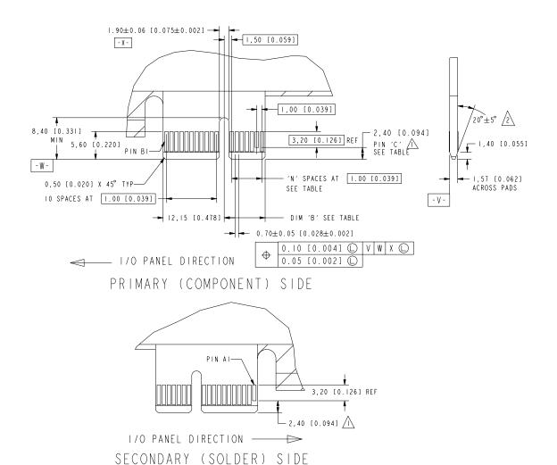
NO TIE BAR PERMITTED FROM CARD EDGE TO LEADING EDGE OF PAD FOR PINS AL AND 'C'.
