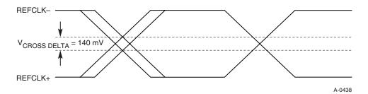
Figure 2-4: Single-Ended Measurement Points for Delta Cross Point
