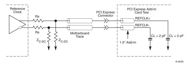
Figure 2-9: Reference Clock System Measurement Point and Loading
