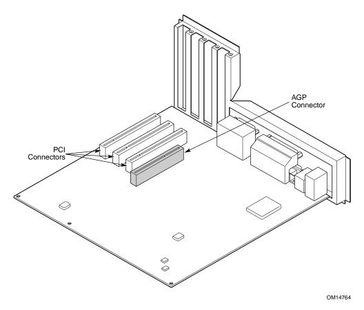
Figure 6-10: Example of a PC System in microATX Form Factor
