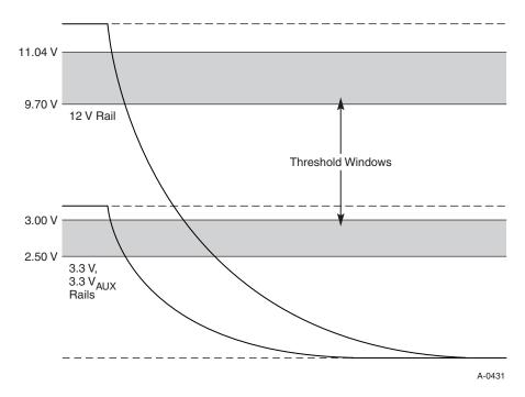
Figure 2-12: Out-of-tolerance Threshold Windows
