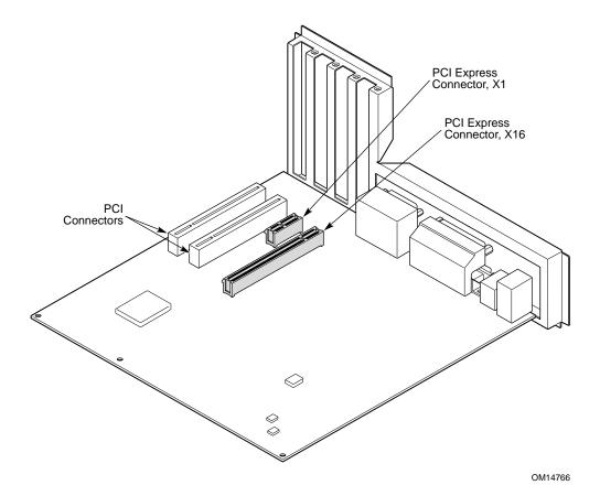
Figure 6-12: More PCI Express Connectors are Introduced on a microATX System Board
