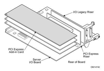
Figure 1-2: Example Server I/O Board with PCI Express Slots on a Riser
