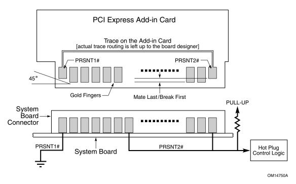
Figure 3-1: Presence Detect in a Hot-Plug Environment
