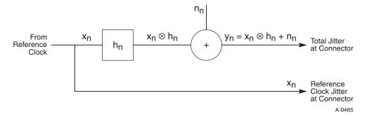
Figure 4-11: Two-Port Measurement Model
