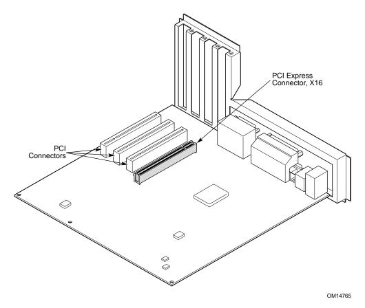
Figure 6-11: Introduction of a PCI Express Connector in a microATX System
