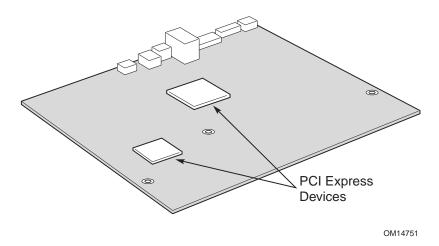
Figure 4-1: PCI Express on the System Board
